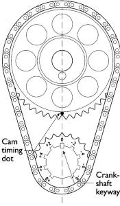
1. Before assembly carefully inspect the crankshaft sprocket. Note the position of each keyway on the inside diameter and the position of the equivalent timing mark on the outside gear tooth.
