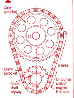
Rotate engine until No. 1 piston is Top Dead Centre (T.D.C.) on compression stroke. No. 1 piston is located at front of the engine on driver's side. Assemble crankshaft sprocket, camshaft sprocket and chain so that zero timing dots are positioned as shown above. (9 links between dots.)
